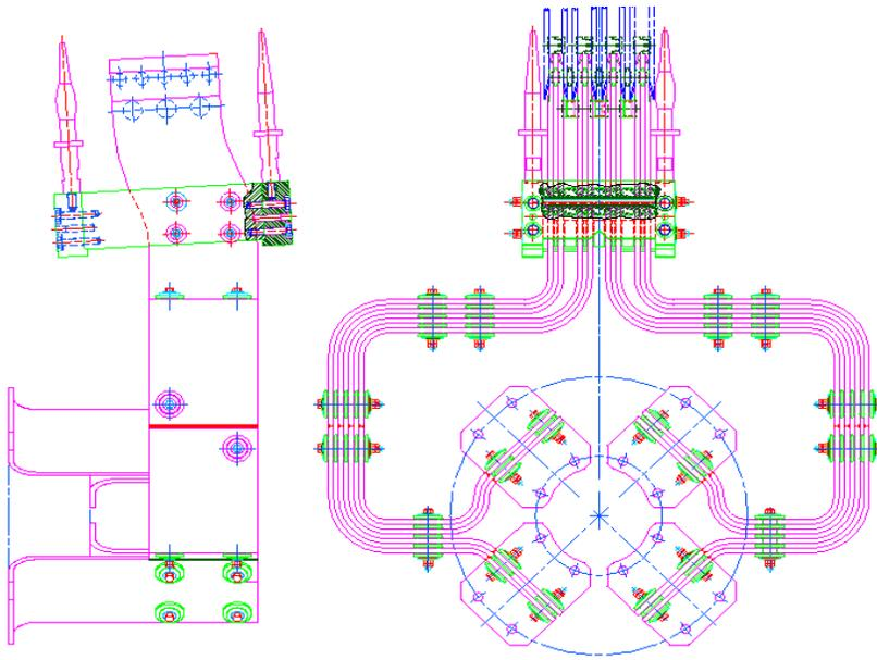
Figure 4.3-13: **Horn 1 Joint Cross Section and Elevation**
