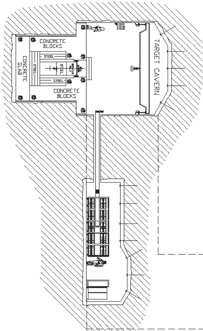
**Figure 4.3-9:** Target Hall and Power Supply Room Cross Section Conceptual Drawing
