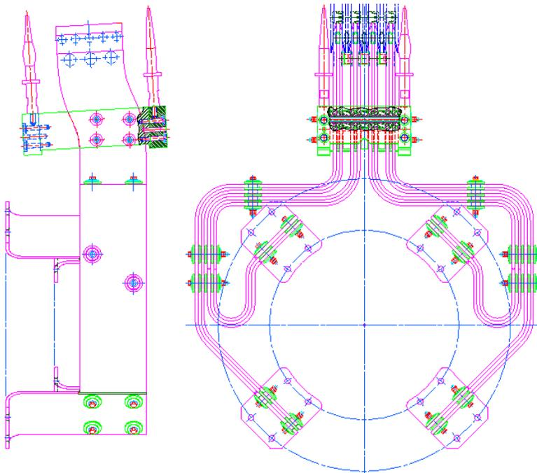
Figure 4.3-14: **Horn 2 Joint Cross Section**
