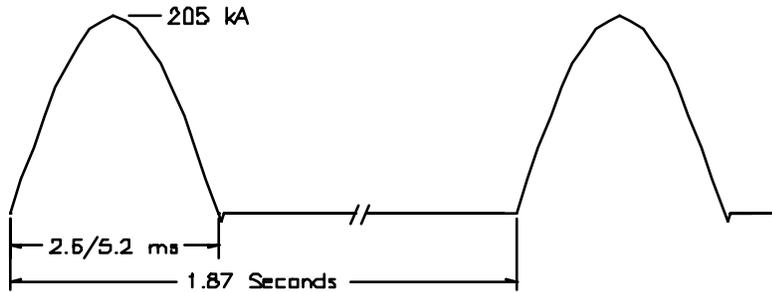
**Figure 4.3-5:** Capacitor Bank Pulse Train Waveform
