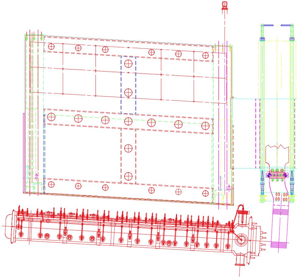
**Figure 4.3-12:** Horn, Remote Clamp and Transmission Line Cross Section
