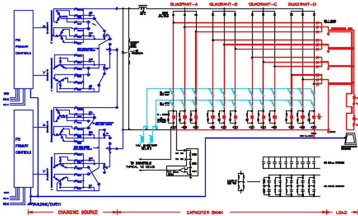
Figure 4.3-4 Horn Power Supply system schematic diagram.
