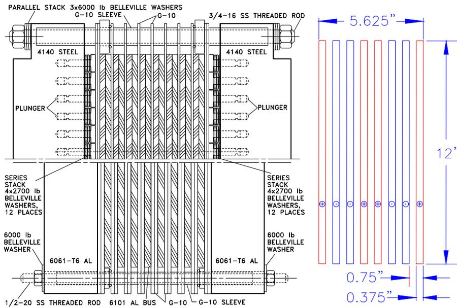
Figure 4.3-8: Stripline Drawing and Pictorial Cross Section.
