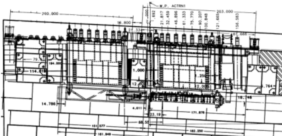
**Figure 4.2-19** Modules in target hall shielding. Target/baffle carrier mounted below target/baffle module, with target and baffle extended into the low energy position. Also visible are carriage cross beams, steel shielding, horn 1 mounted below horn 1 module.
