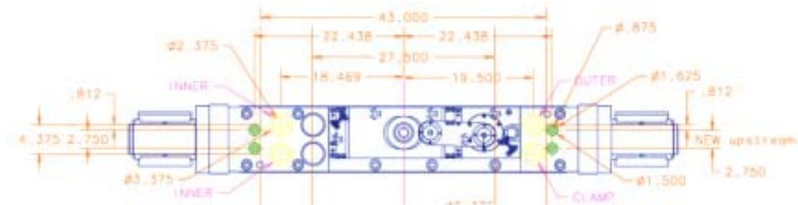
**Figure 4.2-24** Top view of Horn 1 module upstream endwall, which will be copied for the target module. Utility penetrations include those labeled clamp, outer, inner, and the two large holes to the right of those labeled inner.
