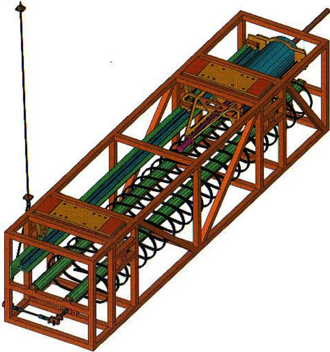
**Figure 4.2-20** Target/baffle carrier with target and baffle mounted. Target shown extended into the low energy neutrino beam position
