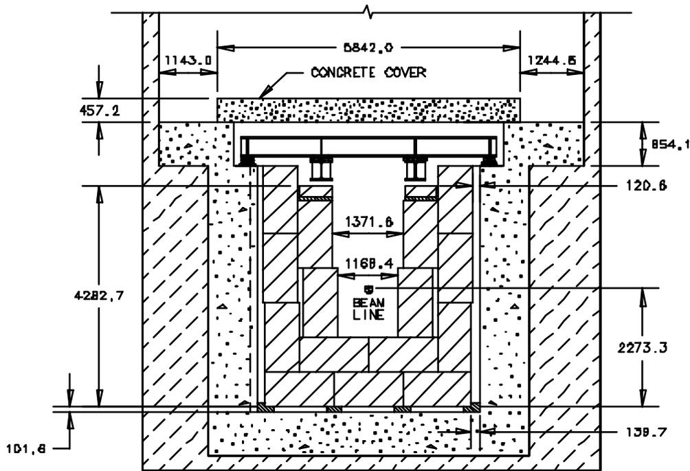
**Figure 4.2-37** Steel walls and floor, concrete shielding
