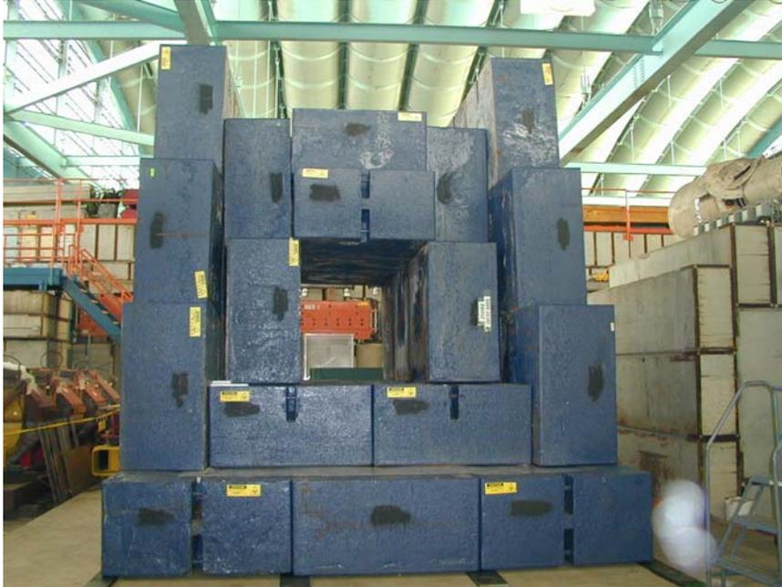
**Figure 4.2-39** Steel shielding downstream of horn 2
