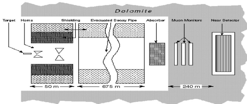
**Figure 2-1** Schematic drawing of the NuMI neutrino beam-line
