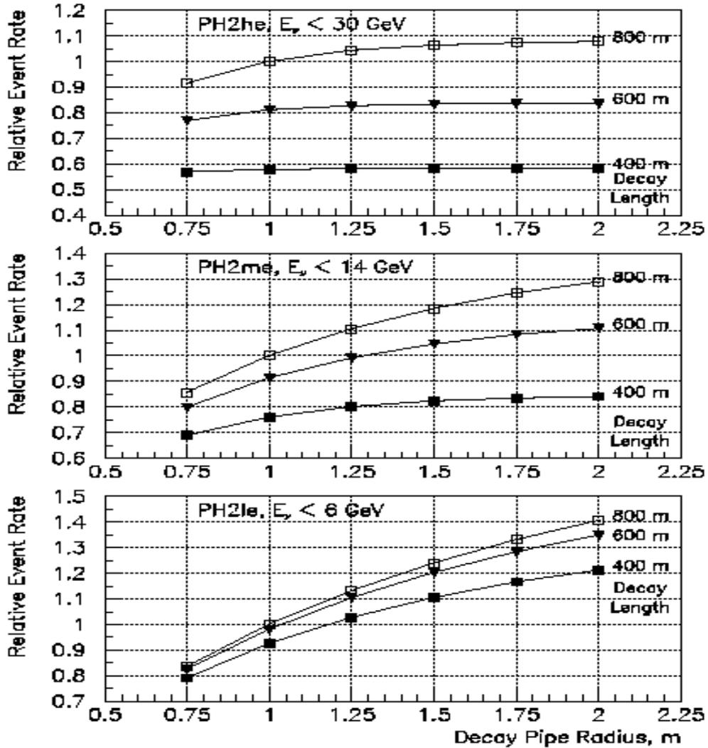
Figure 2-9 Comparison of neutrino event rates as a function of decay pipe length and radius.
