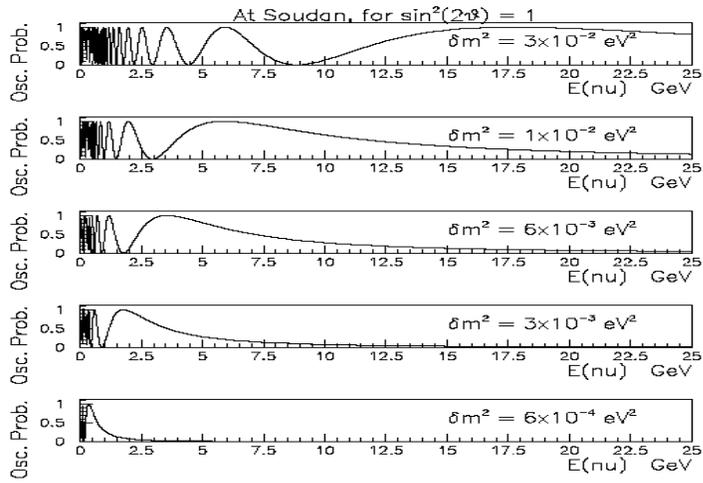
**Figure 2-2** Neutrino oscillation probability as a function of energy for values of  $\Delta m^2$  covering the region appropriate to the atmospheric anomaly.
