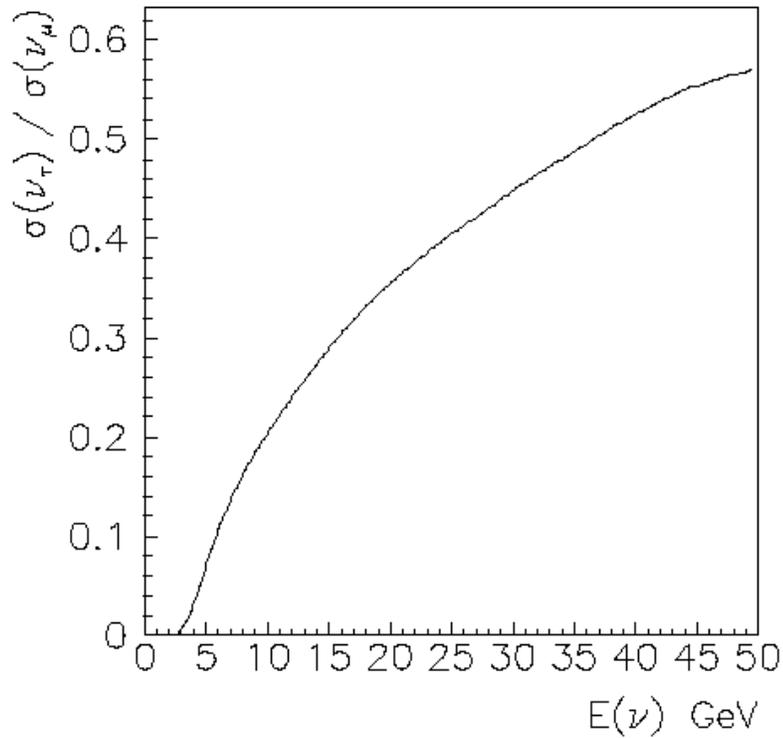
**Figure 2-4** The ratio of the  $\nu_\tau$  charged current interaction cross section to the  $\nu_\mu$  charged current interaction cross section, plotted as a function of neutrino energy.
