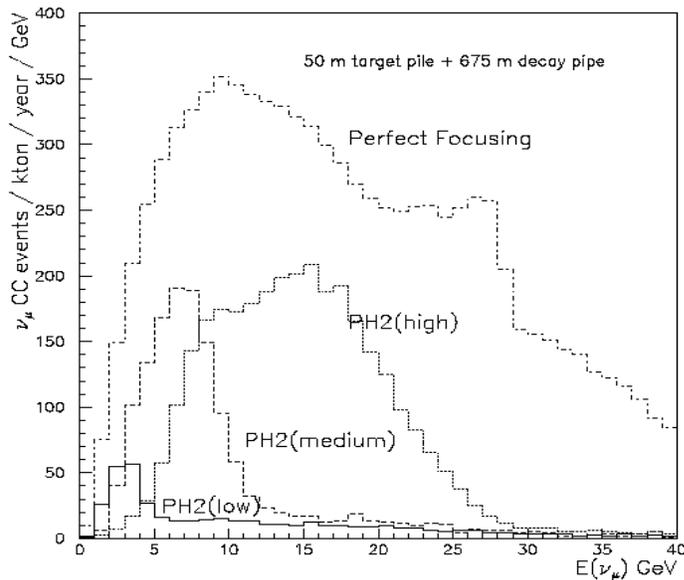
**Figure 2-5** Comparison of event rates at Soudan in the case of ideal perfect focusing, and rates achieved with three configurations of the PH2 beam design.
