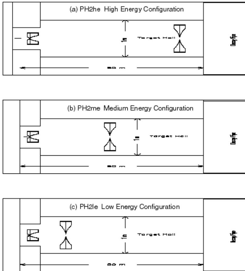
**Figure 2-8** Schematic drawing of PH2 beam focusing configurations in the NuMI target hall. To change the tune to lower energy, the target is moved closer (and finally into) the first horn, and the horns are moved closer together
