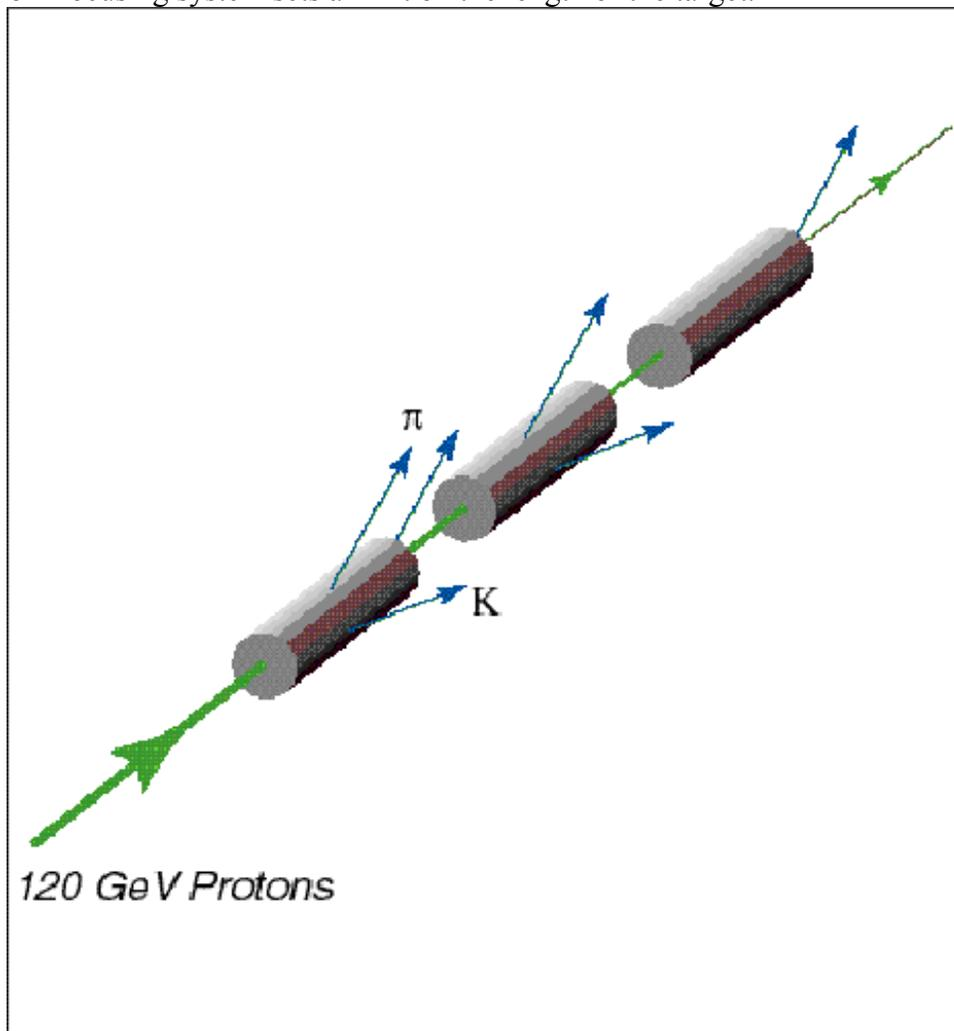
**Figure 2-7** Schematic drawing of a long, slim segmented target for optimum production and decay of pions
