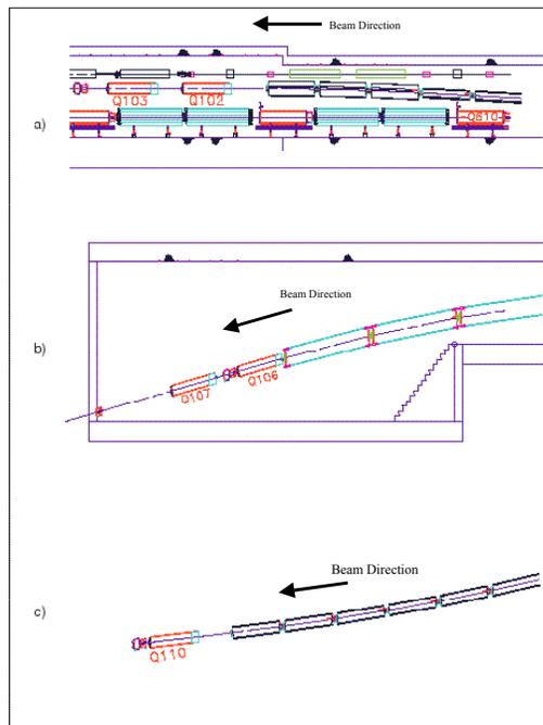
**Figure 2-6** Schematic elevation view of the NuMI primary beam in a) Main Injector enclosure, b) NuMI stub, and c) pretarget hall.
